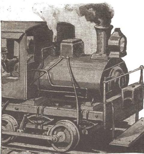
**O**UT of the casual meeting just described was born the “Bell locomotive” which, for a dozen years, was to be a sturdy cart-horse of the construction industry; a geared engine which differed from the Shay, the Climax and the Heisler by adding moderately high speed to impressive tractive effort.
