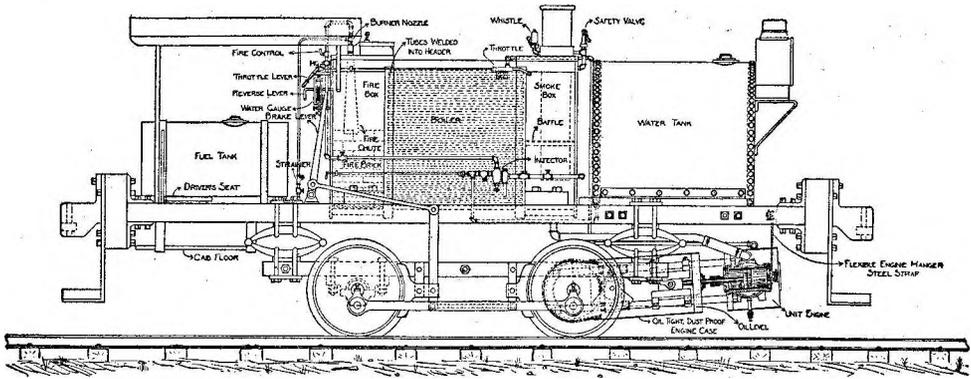
**STANDARD BELL ENGINE DESIGN, showing general arrangement of parts.**
